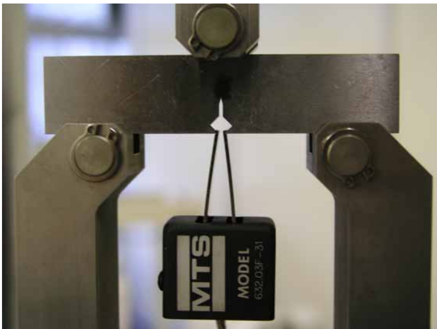
Figure 3-4 0.4T SE(B) Specimen and Clip gage
