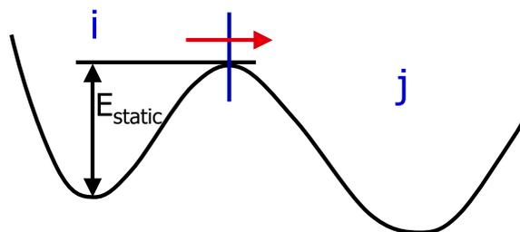
**Fig. 3.** Illustration of the transition state theory rate constant. The unimolecular rate constant for escape from state  $i$  to state  $j$ ,  $k_{ij}$ , is given by the equilibrium outgoing flux through the dividing surface separating the states.
