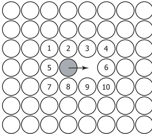
**Fig. 4.** Schematic illustration of the rate catalog concept for the diffusional jump of a vacancy. Atoms in the lattice sites labelled 1-10 can affect the rate constant significantly, so TST rate constants are computed for all possible occupations (differing atom types or vacancies) of these sites. This list of rates makes up a *rate catalog*, which can be accessed during the KMC simulation to determine the rate constant for the jump of a vacancy in any direction for any environment.
