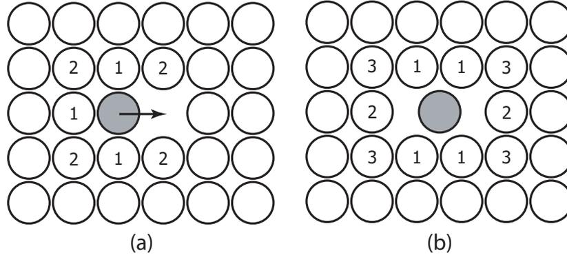
**Fig. 5.** Schematic illustration of the additive rate catalog for the diffusive jump of a vacancy. Sites are labeled by class for (a) the minimum and (b) the saddle point.
