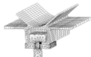
(c) 3D Solid Model for the Analysis of Bolt Axis (8924 nodes, 9708 elements)
