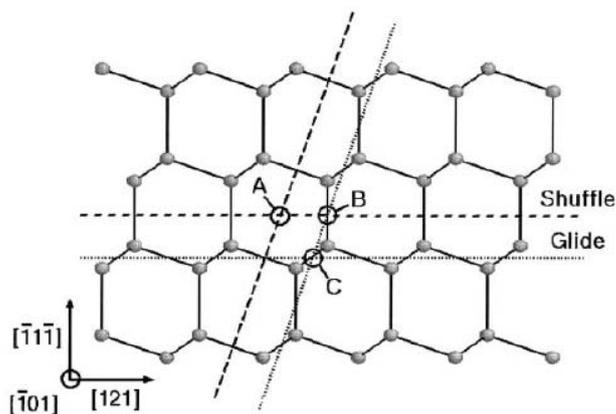
Figure 2. Ball-and-stick representation of the  $(\bar{1}01)$  plane of the cubic diamond structure. The three circles A, B and C indicate the positions of the dislocation line. Broken (dotted) lines show the 'shuffle' ('glide')  $\{111\}$  planes.
