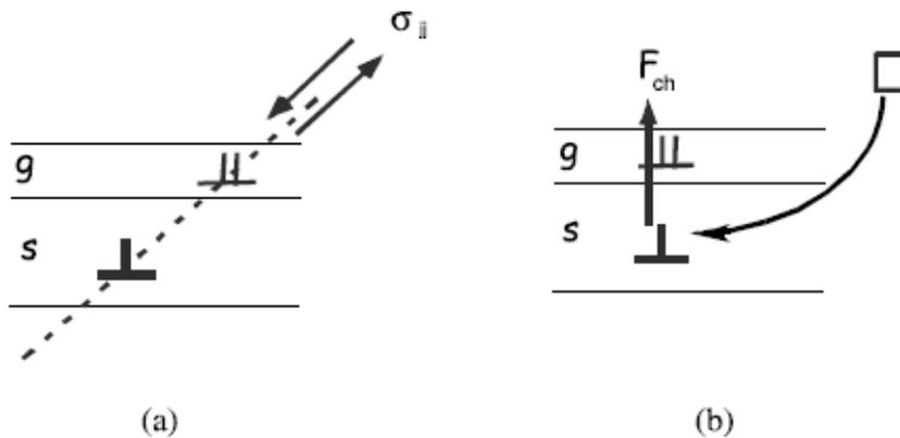
**Fig. 3** Transformation from a perfect shuffle into a dissociated glide. The perfect dislocation has moved from one atomic plane in the glide set by: a) cross slip under the action of a mechanical force and b) climb under the action of a chemical force.
