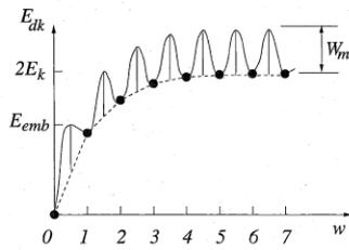
Figure 7-2: Theoretical dependence of the kink pair energy  $E_{dk}$  on its width  $w$  are shown as dots. For large width it approaches  $2E_k$ . At finite width  $w$ ,  $E_{dk}$  is a superposition of  $2E_k$  and the kink pair interaction energy  $W_{int}(w)$ . The solid curve illustrates the energy barrier between the neighboring states.  $E_{emb}$  is the barrier for nucleating an embryonic double-kink, i.e. transition from state  $w = 0$  to  $w = 1$ .
