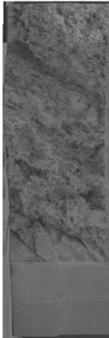
Fig 4.9: Creep fracture surface of test piece of CT ( 800^{\circ}\text{C} )
