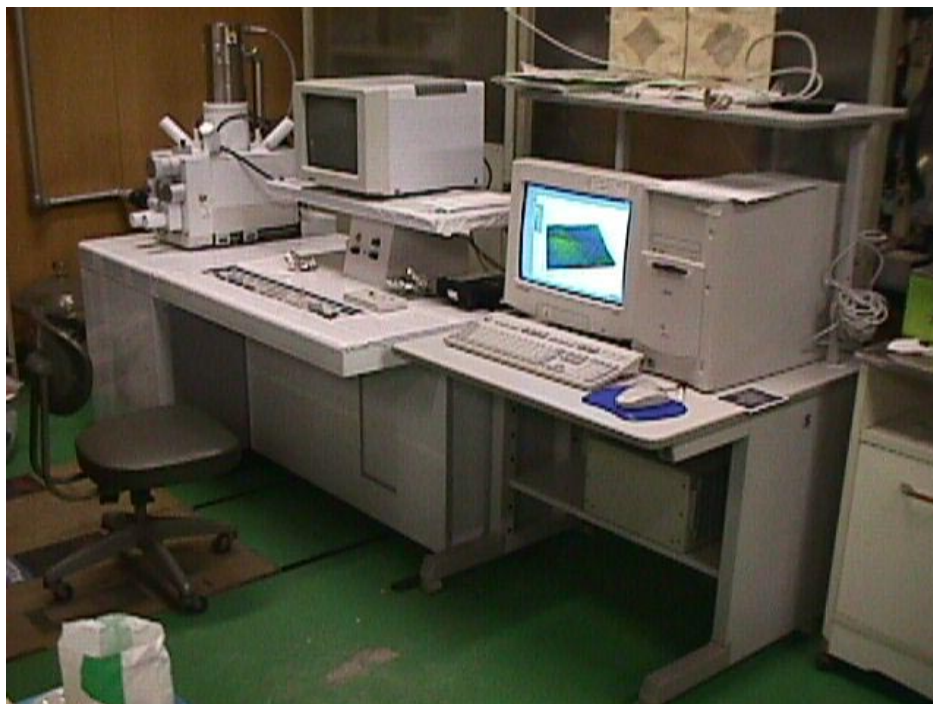
Fig A.1: Appearance of ERA-4000 SEM device
