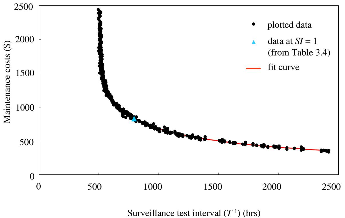
Fig 3.17. Optimal maintenance costs- $T^1$  plot
