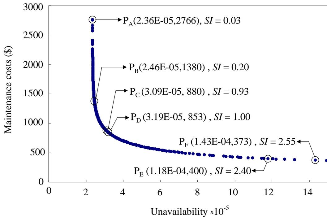
Fig 3.9. The Pareto-optimal solutions for minimization of unavailability and maintenance cost.
