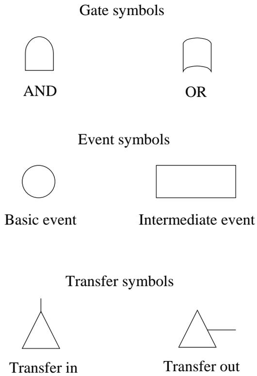
Fig. 2.2. The generally used conventional fault tree symbols.
