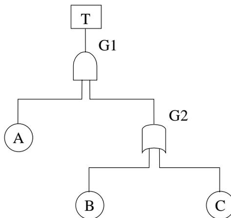
Fig. 2.3. The simple example of a fault tree.
