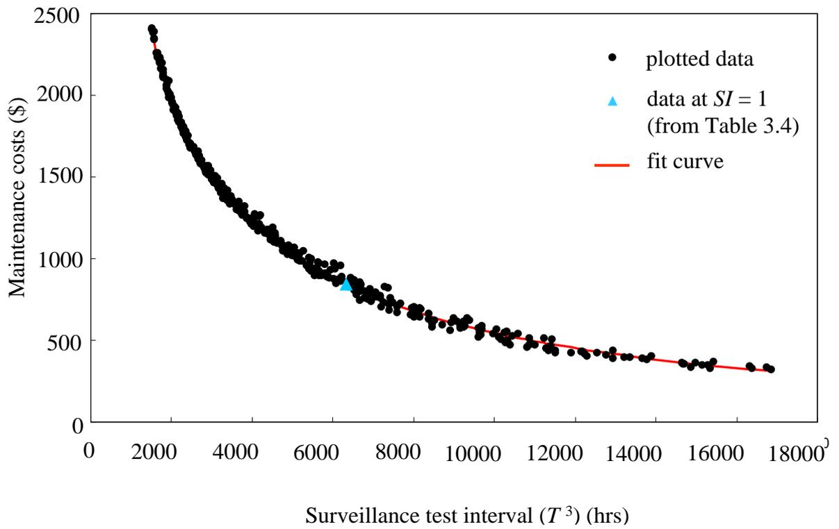
Fig 3.19. Optimal maintenance costs- $T^3$  plot
