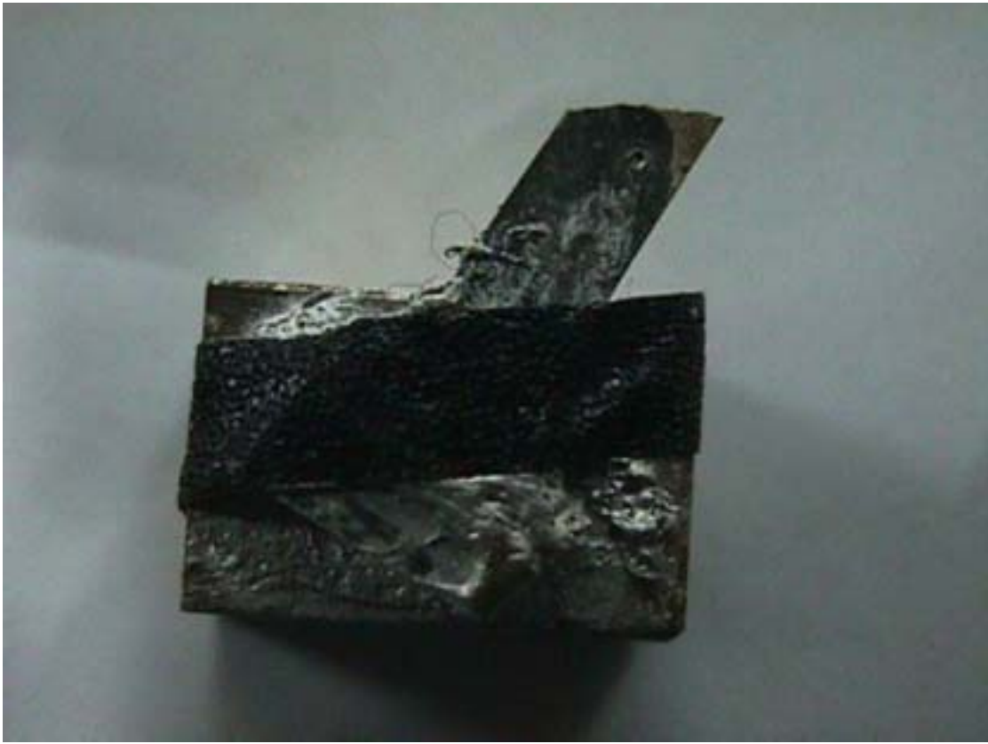
Fig. 5.11: Appearance of test piece of DEN (Creep fatigue)
