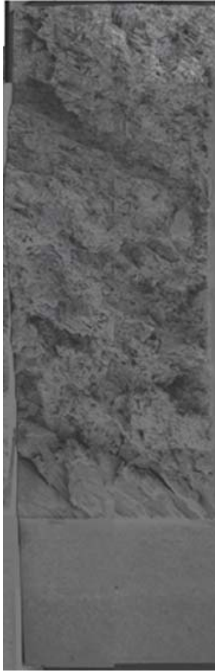
Fig. 5.17: Creep fatigue fracture surface of test piece of CT ( 850^{\circ}\text{C} )
