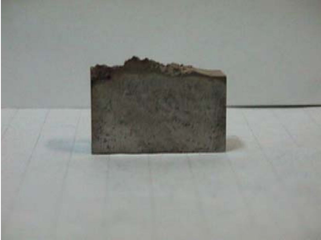
Fig. 5.13: Appearance of test piece of CT ( 850^{\circ}\text{C} )
