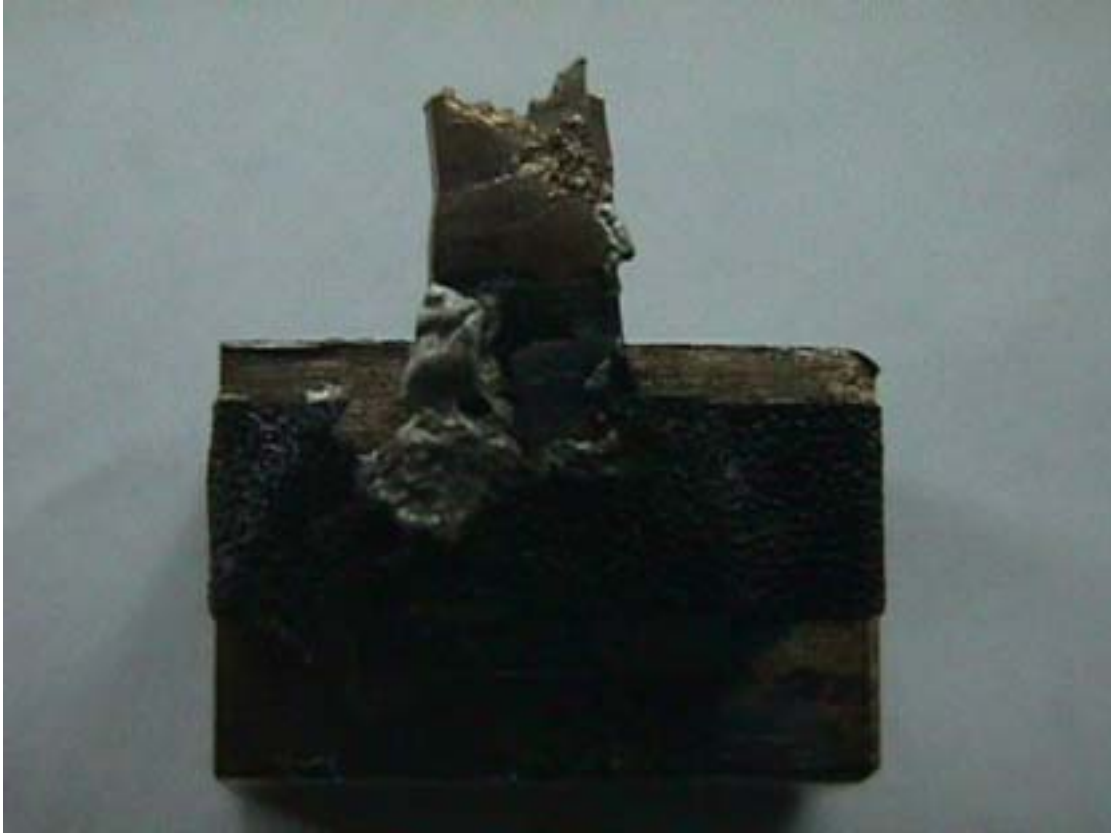
Fig. 5.10: Appearance of test piece of DEN (Creep)
