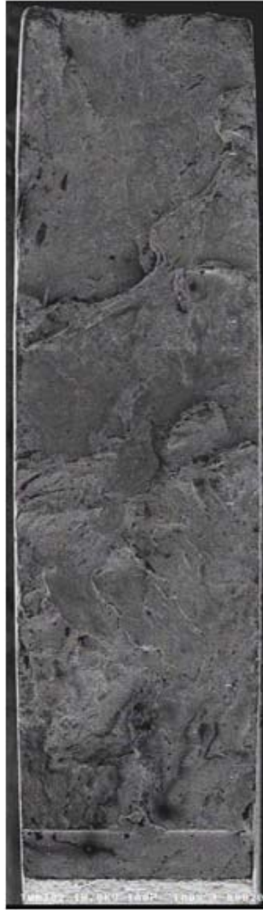
Fig. 5.15: Creep fatigue fracture surface of test piece of DEN
