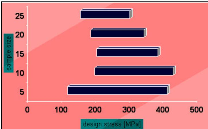
Fig 145: Design stress bounds determined using MLM
