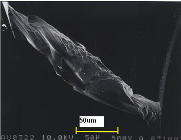
Fig 95: A typical fractured surface for combined loading (note the undulating surfaces and river patterns)
