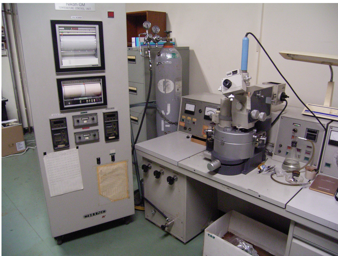
Fig. 3.6 Photograph of hot hardness testing machine, QM
