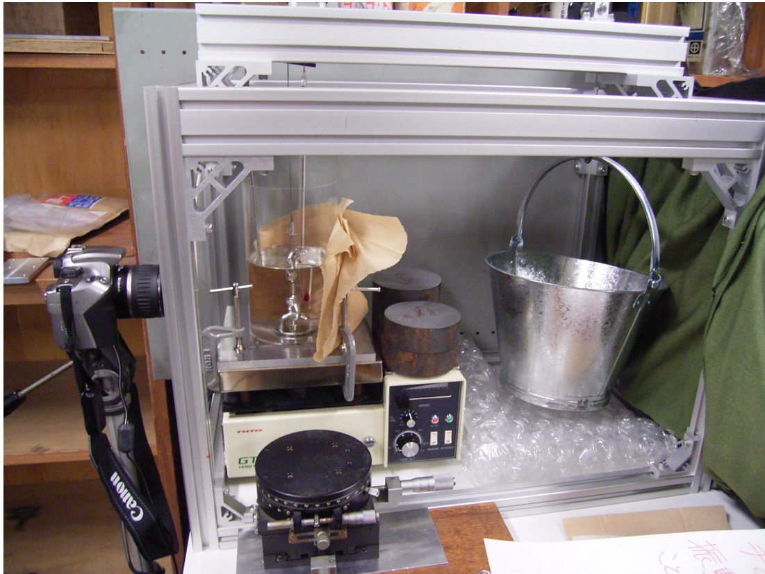
Fig. 3.8 Photograph of tension creep testing machine
