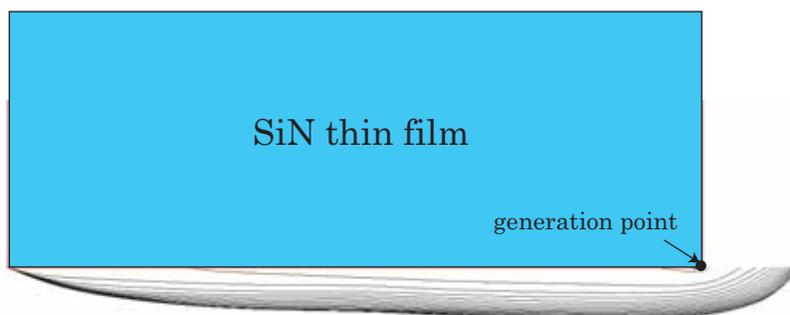
Fig. 3.5 Propagation of a dislocation in the CZ wafer under large share stress caused by the SiN thin film. Snapshots are plotted by the same number of computational step with upside view.
