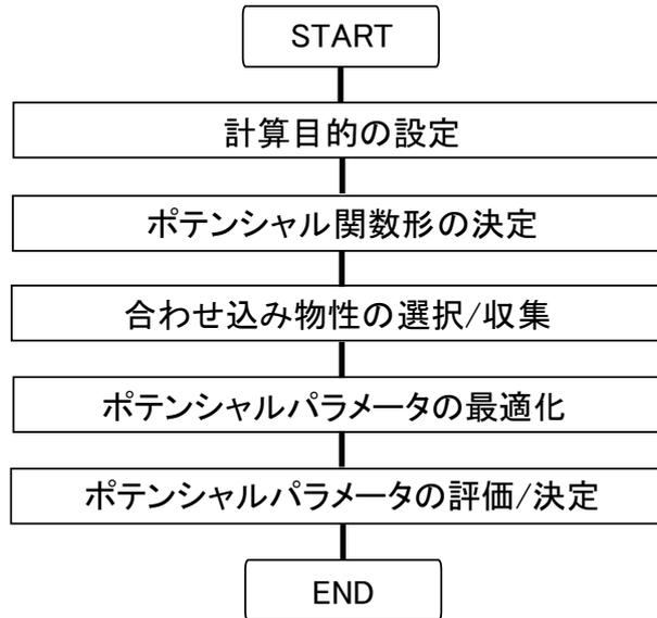
Fig. 3.1: The flowchart for fitting process
