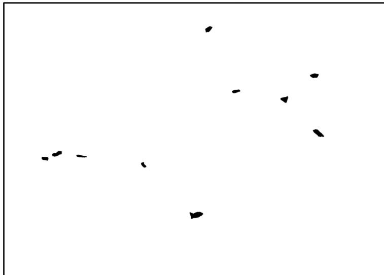
Fig. 3-6 Binarized image of creep voids(Observed area: 93\mu\text{m} \times 69\mu\text{m} ).
