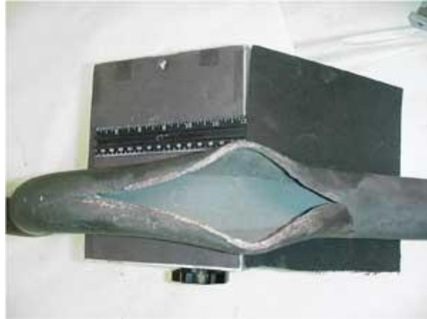
↑ Fig.1.1d Failure by a loss of creep-rupture strength [7]
