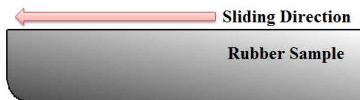
Fig. 3-9 A cross sectional view of edge-processed rubber sample.
