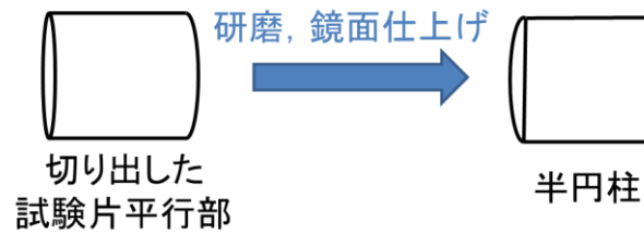
Fig. 2-16 Schematic illustration of polishing of specimens
