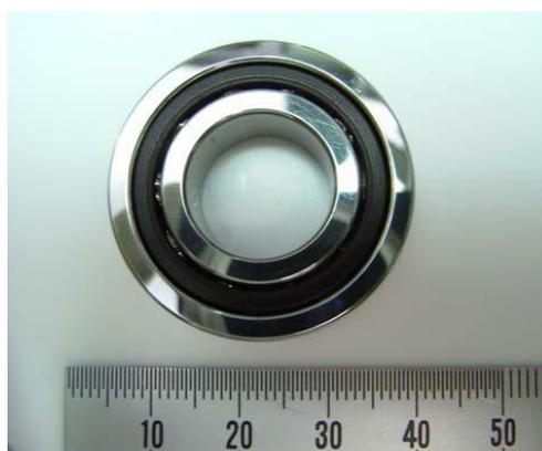
Fig. 3-1 Test bearing
