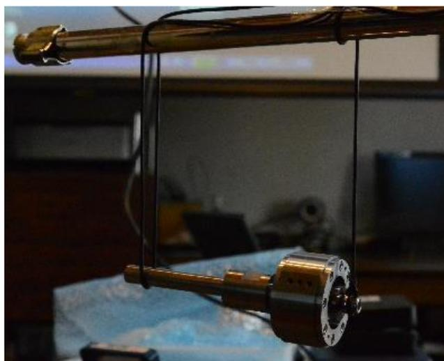
**Fig. 2-2 Test apparatus (both ends free)**
