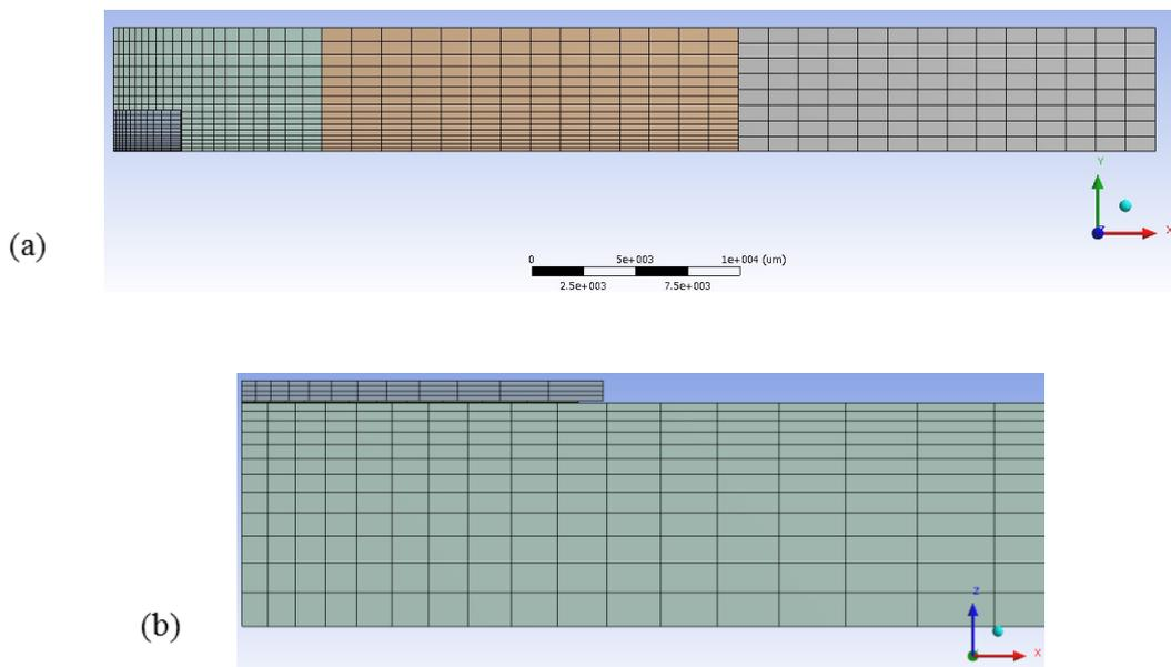
Fig 57. Lateral condition FE Model of four-point bending (a)top view (b)side view.
