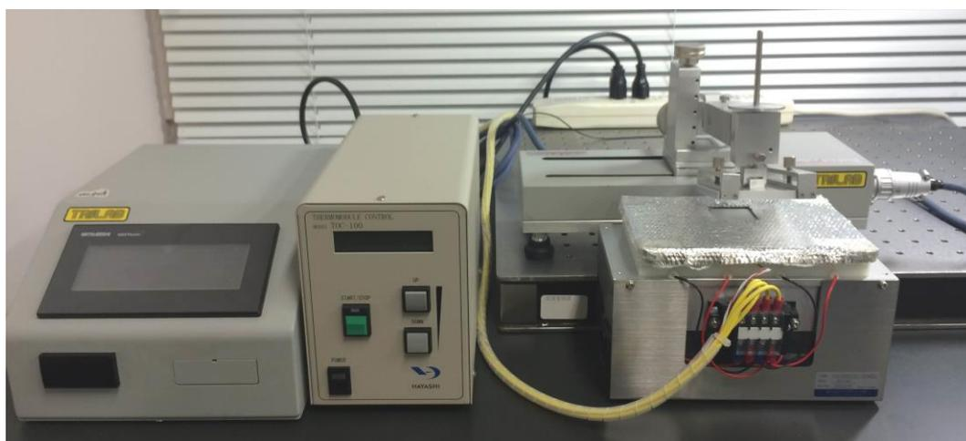
Fig. 5-14 Friction test unit.
