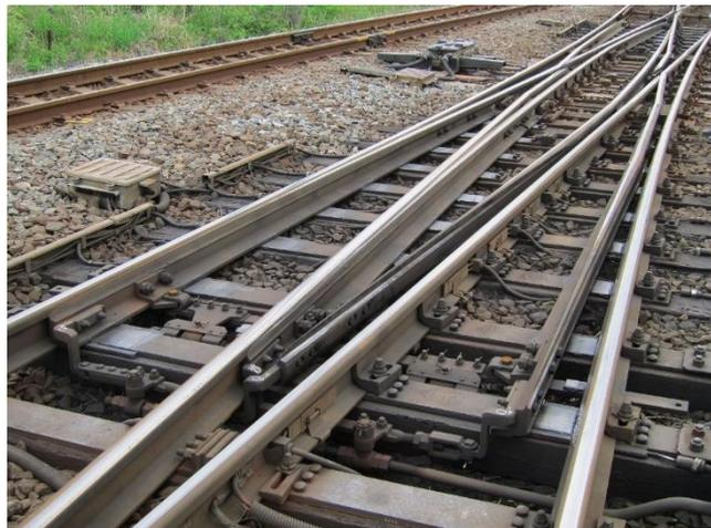
Fig. 2.7 Double slip switch on the track [9].
