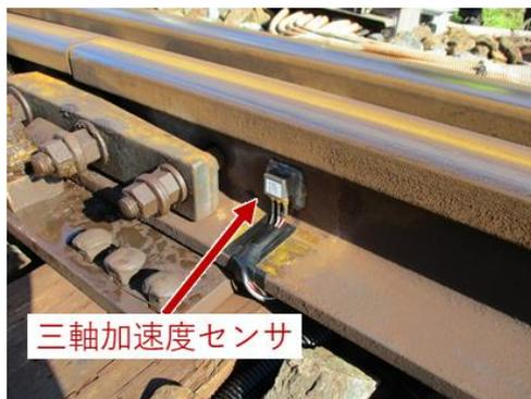
Fig. 3.3 The measuring equipment at the heel of tongue rail.
