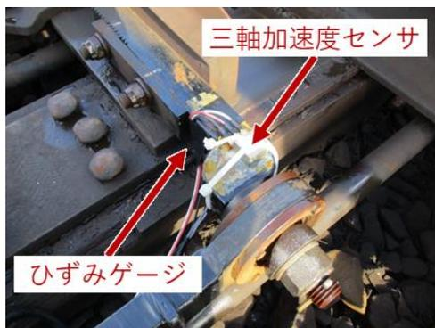
Fig. 3.5 The measuring equipment at the hook of front rod (normal switch).
