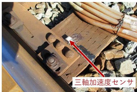
Fig. 3.6 The measuring equipment at the wooden sleeper (normal switch).
