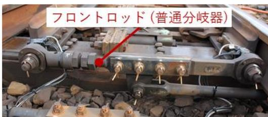
Fig. 2.9 Front rod (normal switch).
