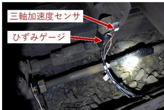
Fig. 3.4 The measuring equipment at the hook of front rod (double slip switch).
