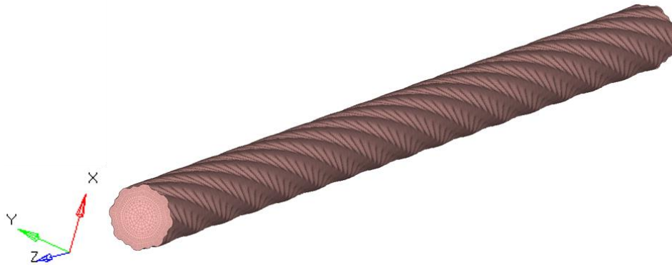
Fig. 3-8 Core model after thermal expansion
