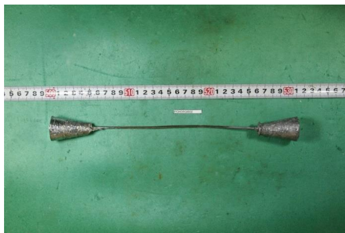
Fig. 2-27 Appearance before the strand tensile test
