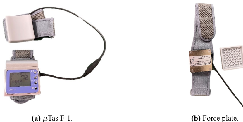
Figure. B-2. Hand-held dynamometer. Isometric muscle strength measurement device \mu Tas F-1 by Anima.
